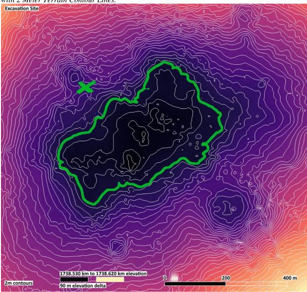
*Figure 3. Excavation Site (outlined in green) and Water Extraction Plant (shown by green X) with 2 Meter Terrain Contour Lines.*
